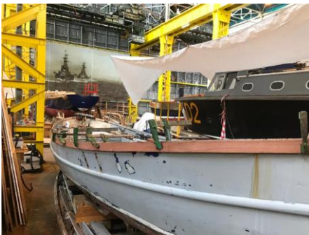
Below left the inserts have been steamed and are drying out in place so that they hold their shape. Below middle you can see the hand of Keiron O as he removes wet and rotten timber from the apron attached to the stern log and finally far right Hamo T is planing off the surplus gunwale inserts after the glue has cured.
