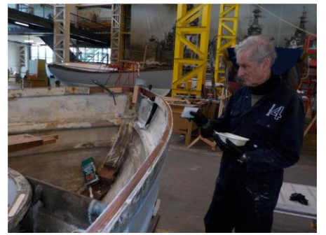
Below left the inserts have been steamed and are drying out in place so that they hold their shape. Below middle you can see the hand of Keiron O as he removes wet and rotten timber from the apron attached to the stern log and finally far right Hamo T is planing off the surplus gunwale inserts after the glue has cured.
