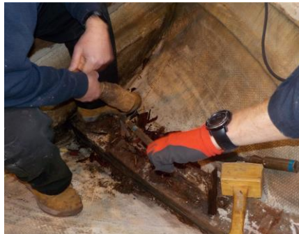
Below left the inserts have been steamed and are drying out in place so that they hold their shape. Below middle you can see the hand of Keiron O as he removes wet and rotten timber from the apron attached to the stern log and finally far right Hamo T is planing off the surplus gunwale inserts after the glue has cured.
